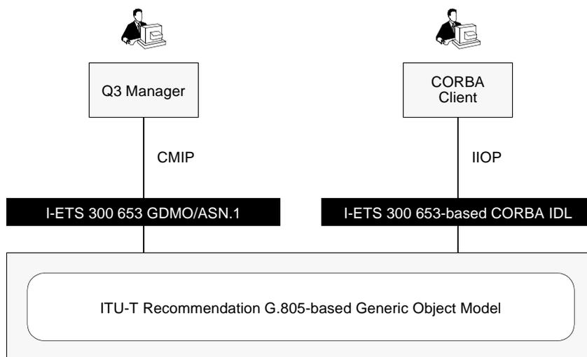
Figure 2: The North-facing Interfaces Provided by the NMS
