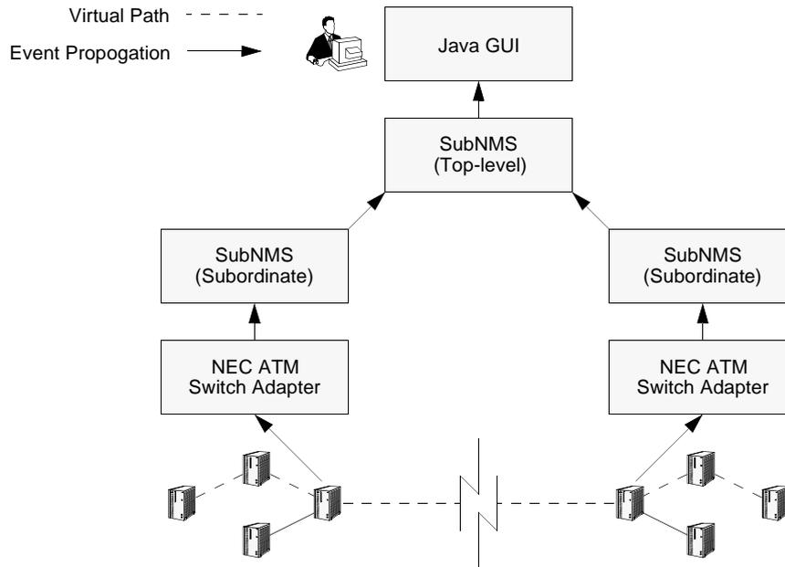
Figure 7: Event Propagation Using the Prototype NMS
