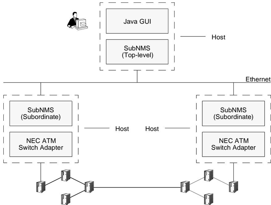
Figure 5: The Prototype NMS Deployed in the Test Network
