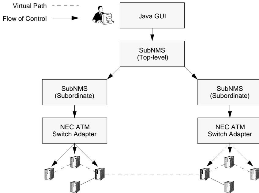
Figure 6: Setting up a VP Using the Prototype NMS
